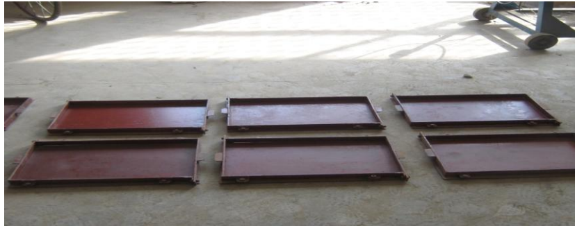
Shrinkage moulds of size 300*500*30mm
