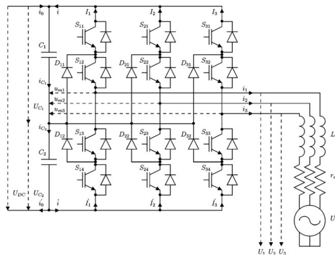
Fig. 4. Schematic of the three-level neutral point clamped converter.
