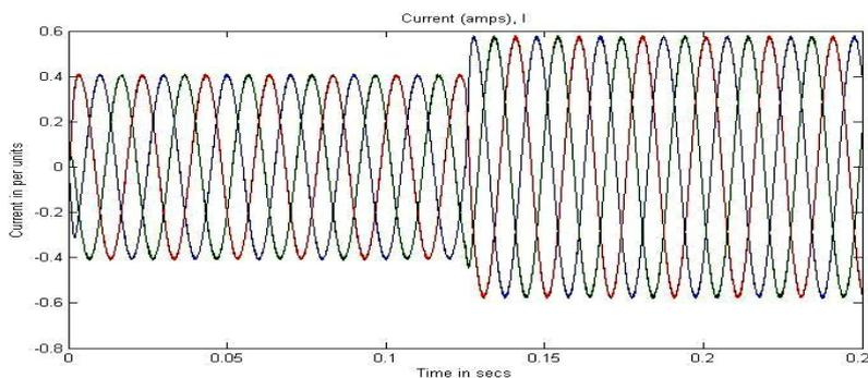
Fig8(c) UPFC series converter controlling real and reactive power flow, comparison between controllers Fuzzy and PI of Shunt converter with DPC controller on series converter under step wise changes.
