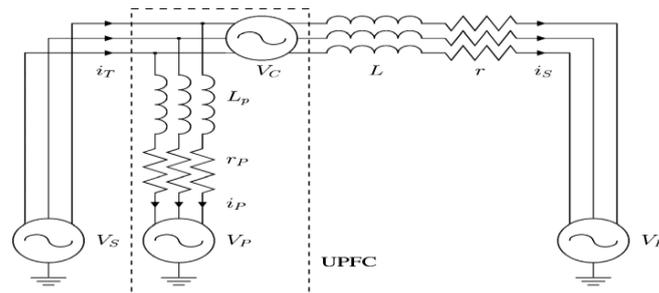
Fig. 3. Schematic of the equivalent circuit of the UPFC system.
