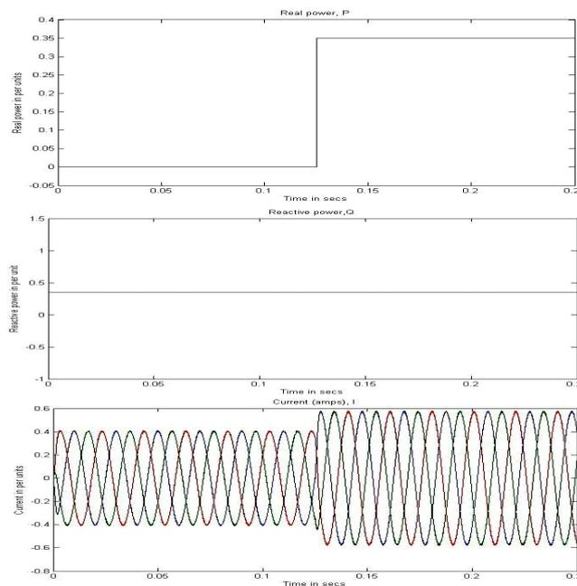
(b) Fig.8:UPFC series converter controlling the power flow under balanced conditions, 250-ms view during stepwise change of active and reactive power flow reference  $P_{ref}, Q_{ref}$  Simulation ( P 948Wpu, Q948 VARpu)
