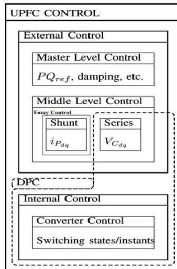
Fig. 2. UPFC controller classification according to [2] and [3], and the position of the proposed direct power controller (DPC).
