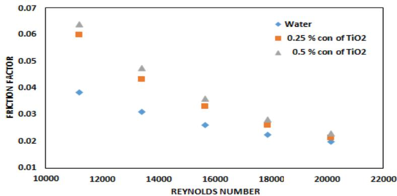
Figure 11: Reynolds number vs Friction factor in plane tube in laminar regime with water and nanofluids
