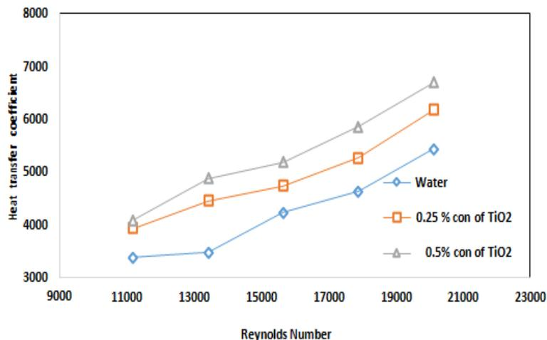
Figure 11: Heat transfer coefficient enhancement in plane tube with nanofluids in turbulent regime.
