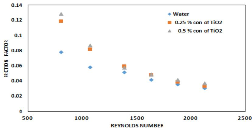
Figure 12: Reynolds number vs friction factor in plane tube in turbulent regime with water and nanofluids
