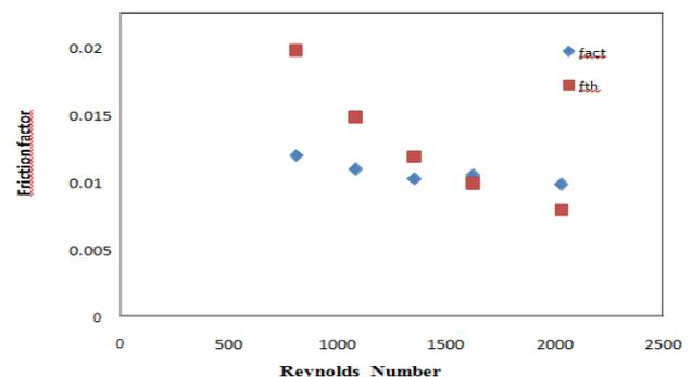
Figure 5: Comparison of Experimental and Theoretical Pressure drop values in Laminar flow
