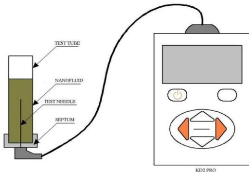
Figure 3: Schematic Diagram of thermal conductivity measurement arrangement
