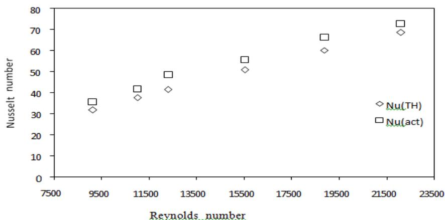
Figure 6: Comparison of Experimental and Theoretical Nusselts values
