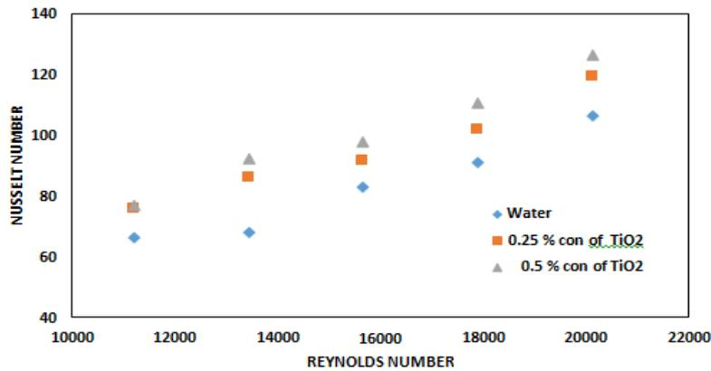
Figure 9: Reynolds number vs Nusselt number in plane tube in turbulent regime with water and nanofluids. The figure 6 shows that show the experimental results for the laminar flow showed average enhancements of 30.66%, and 35.8% for 0.25% and 0.5% of nanofluids compared to Plain tube with water. The figure 5.4 shows that show the experimental results for the turbulent flow showed
