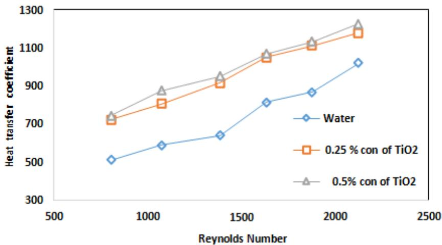
Figure 10: Heat transfer coefficient enhancement in plane tube with nanofluids in laminar regime
