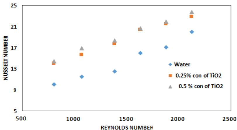
Figure 8: Reynolds number vs Nusselt number in plane tube in laminar regime with water and nanofluids
