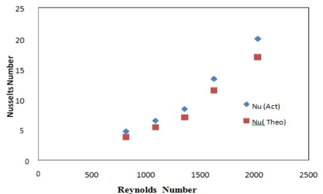
Figure 4: Comparison of Experimental and Theoretical Nusselts Number values in Laminar Flow
