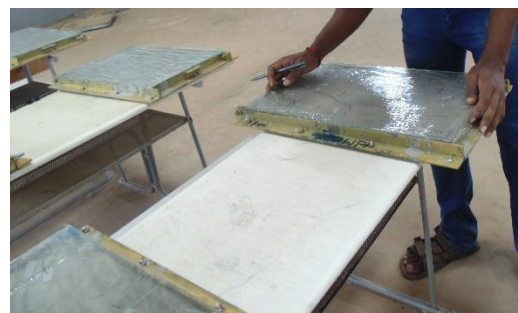
Marking of Cracks
