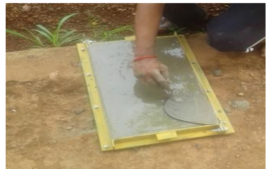
Slurry infiltrated into mould
