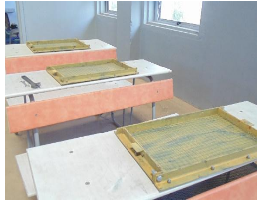
Aligned Mould for Casting the specimen
