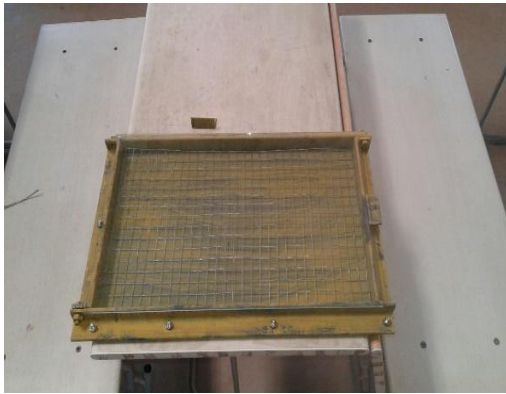
Mould size of 300x500x30mm
