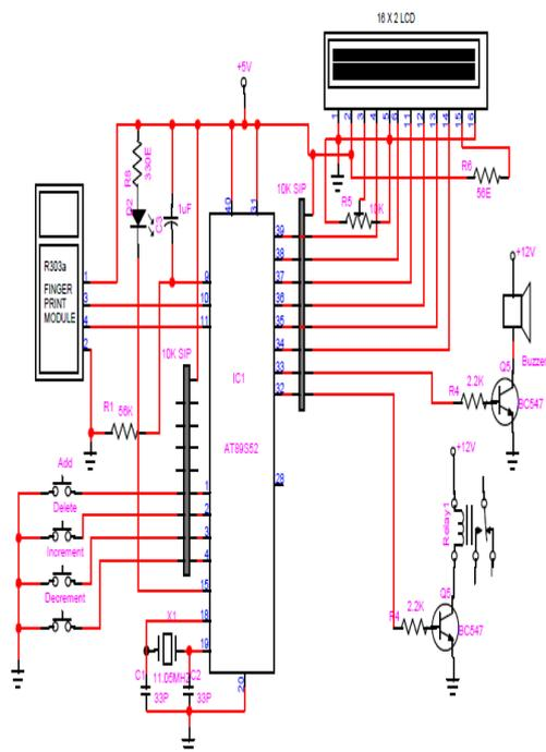
**Fig 2: Biometric Module Interfacing**
