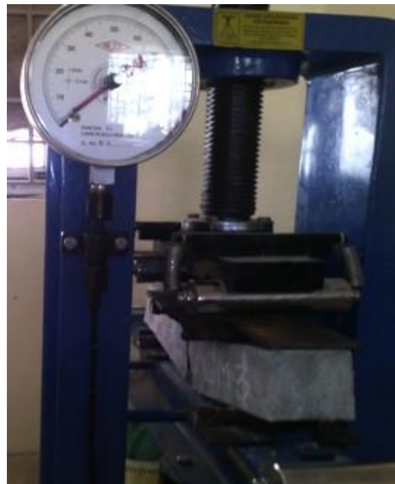
Figure: 4 Failure modes of beams in four point bending
