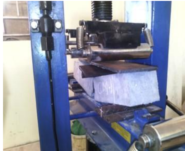
Figure: 3 Failure modes of beams in three point bending
