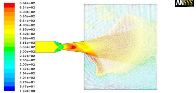
Velocity Vectors Colored By Velocity Magnitude (m/s) ANSYS FLUENT 12.0 (2d, dbns imp, lam) Apr 17, 2015
