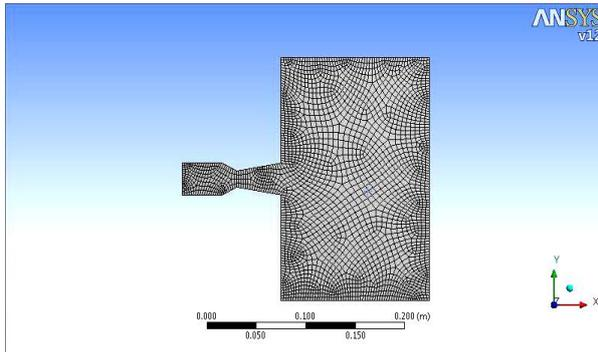
Fig.5. Grid system in C-D nozzle with domain.
