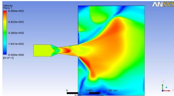
Fig.7. Velocity plane of C-D nozzle.
