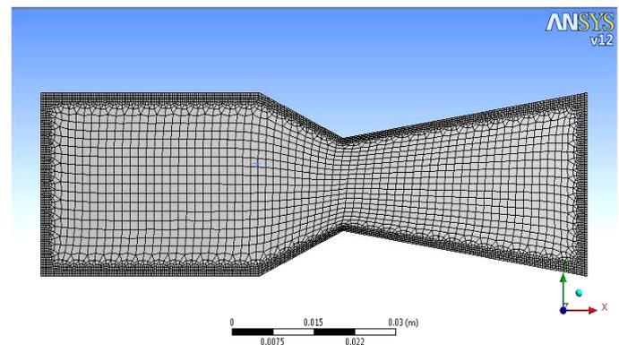
Fig.4. Grid system in C-D nozzle
