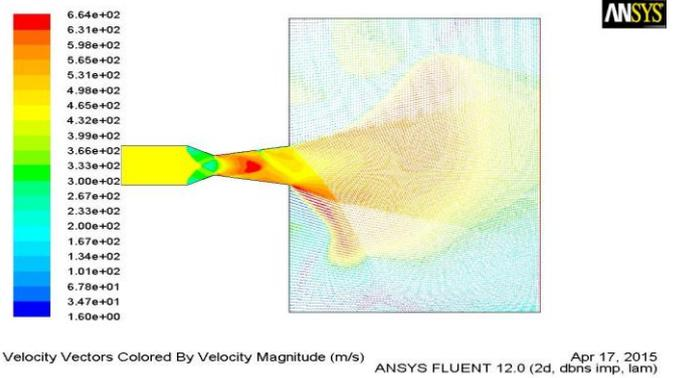
Fig.8. Velocity streamline of C-D nozzle.
