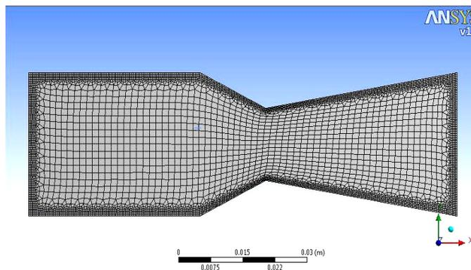
Fig.4. Grid system in C-D nozzle
