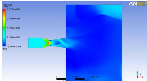
Fig.6. Pressure plane of C-D nozzle.
