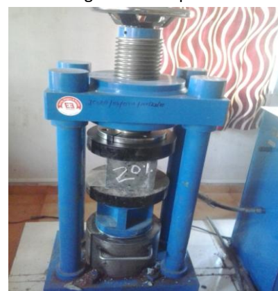
FIGURE 1: COMPRESSIVE STRENGTH TEST SETUP
