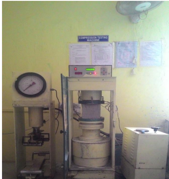
Fig 2: Testing of Cube on Compression Testing Machine
