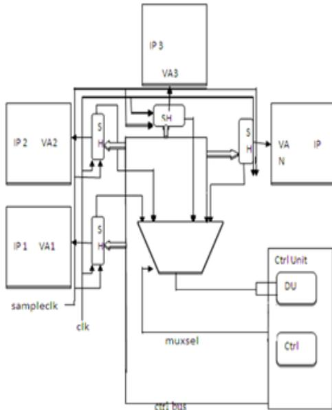
**Figure1: Analog BIST architecture using sampling head technique**
