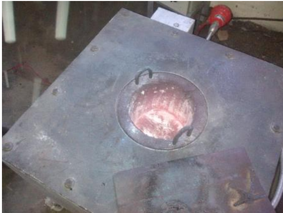
Fig3: Experimental setup of stirring mechanism for the fabrication of MMC.
