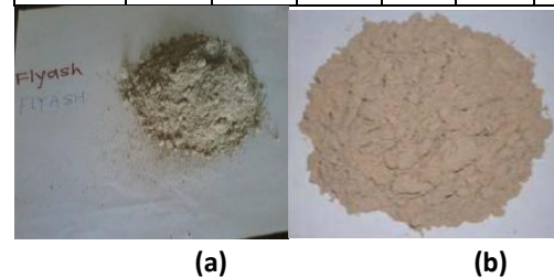
Fig1: The fly ash powder used (a) as received condition (b) After heat treatment condition
