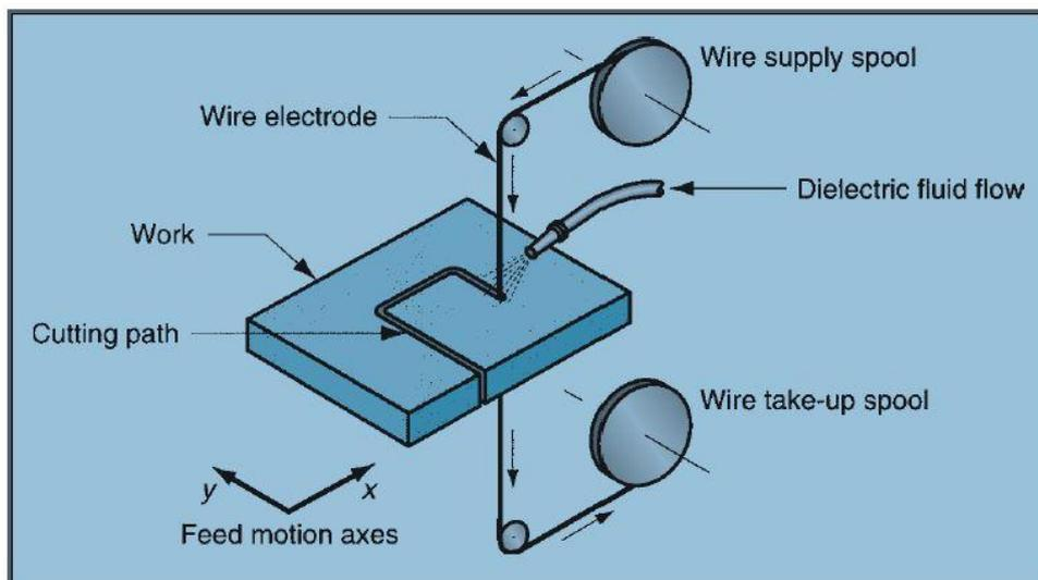
Fig- Wire Electrical Discharge machining process
