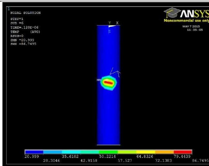
Fig- Temperatur distribution in Tungstenwire with V= 28, I=30A, P=0.35, ton=0.06 $\mu$ s
