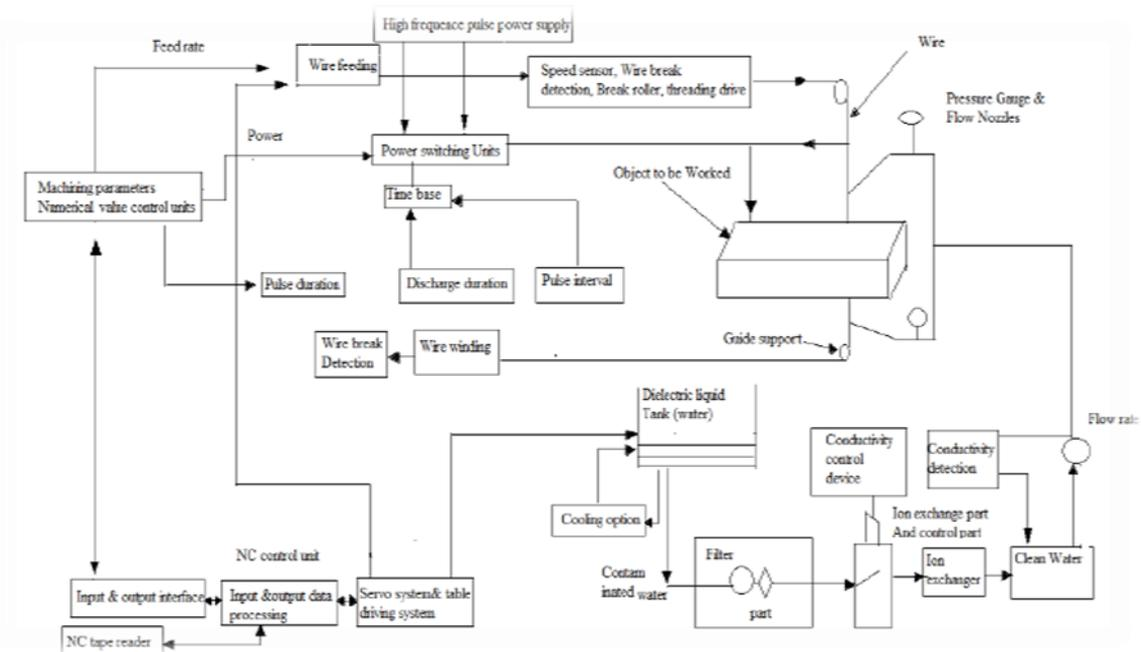
Fig-Schematic diagram of WEDM (Source: Dutta and Mahapatra)
