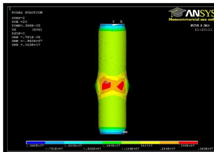
**Fig- Thermal stress in X-component atton=0.12 μs**
