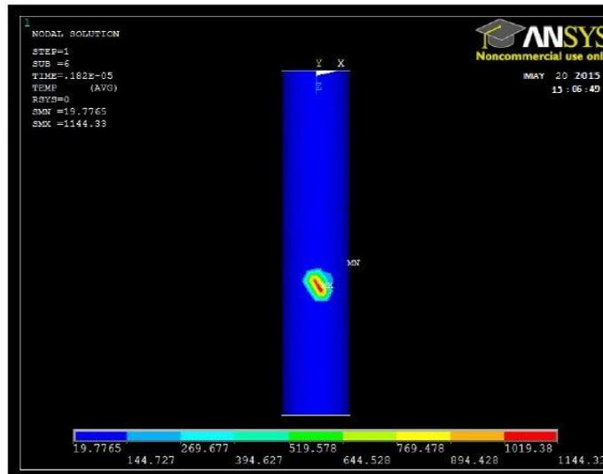
Fig- Temperatur distribution in Tungstenwire with V= 28, I=30A, P=0.35, ton=1.82 $\mu$ s
