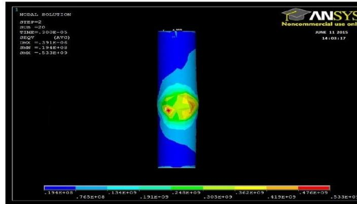
Fig- Residual stress at , ton=3  $\mu$ s
