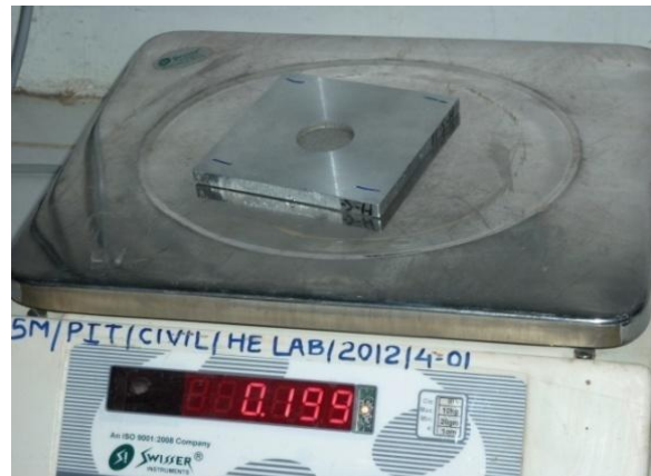
Fig:6 Weight measurement of work piece ROC = \frac{Dia\ of\ the\ work\ piece\ cavity - Dia\ Of\ the\ tool}{2}
