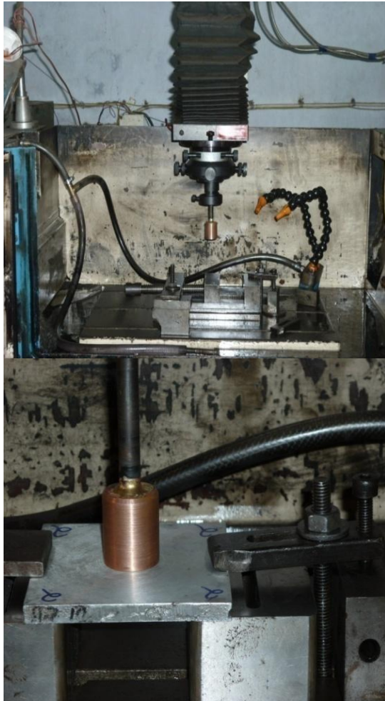
Fig: 3 Tool with tool holder and work piece
