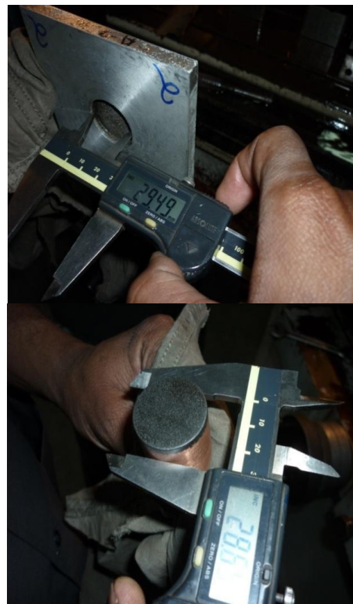
Fig:7 diameter measurement of the tool and work piece
