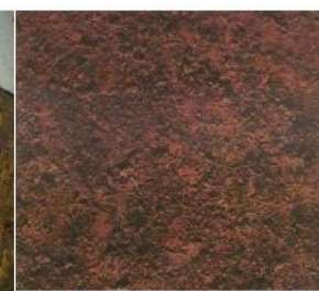
Fig.4- RUST GRADE D
