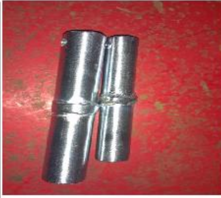
Fig.6- Galvanized material. before test
