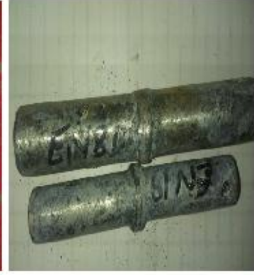
Fig.7-Galvanized material after test.
