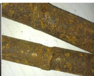
Fig.3- After salt spray test
