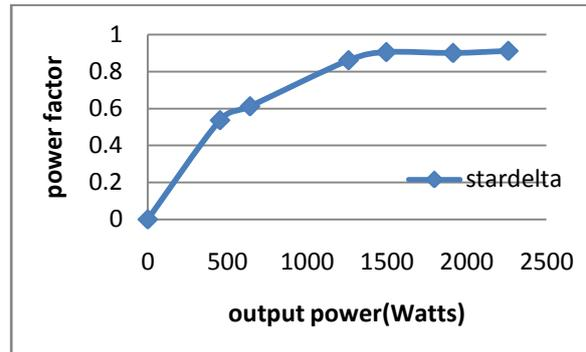
Figure.3.6.Power Factor as a Function of Output Power – Star delta
