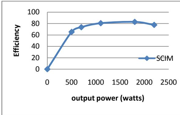
Figure.4.1 Efficiency Vs Output Power – SCIM
