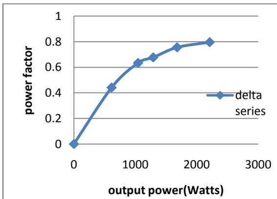
Figure.3.5.Power factor as a function of output power – Delta series
