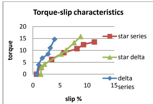
Figure.3.7. Torque Slip Characteristics – MFIM
