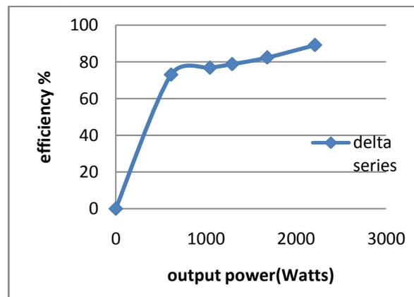
Figure.3.3. Efficiency as a Function of Output Power – Delta Series
