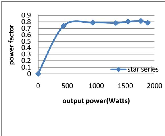
Figure.3.4.Power Factor as a Function of Output Power – Star Series
