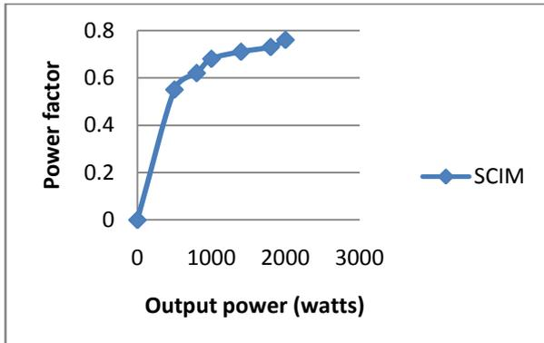
Figure.4.2 Power Factor Vs Output Power – SCIM
