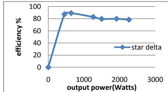
Figure.3.2. Efficiency as a Function of Output Power – Star delta
