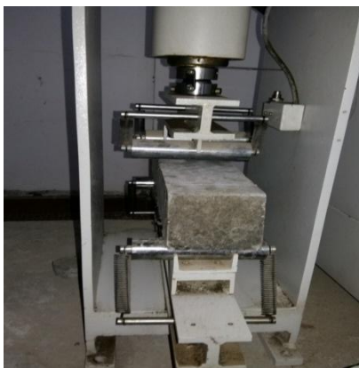
Fig 2. Test setup for flexural strength
