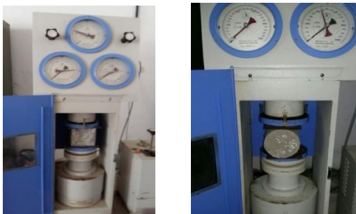
Fig 1. Test setup for compressive strength and split tensile strength respectively.
