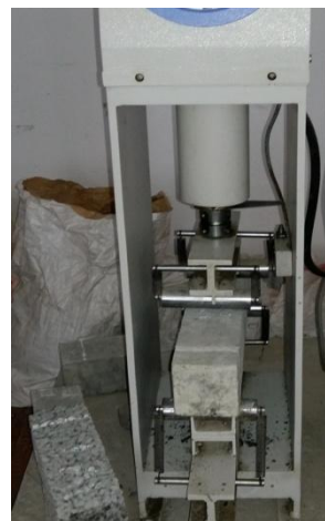
Fig 2. Test setup for flexural strength
