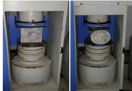
Fig 1. Test setup for compressive strength and split tensile strength respectively.
