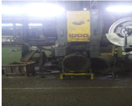
Figure.1 Pneumatic forging press (1000 ton)
