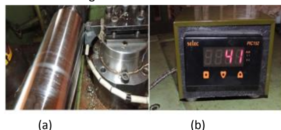
Fig. 4 Temperature measurement set-up (a) Thermocouple ( b) Temperature recorder.
