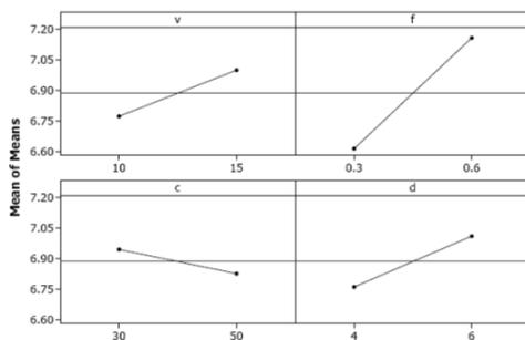
Figure 5.3: Main effect Plot for over cut-depth.
