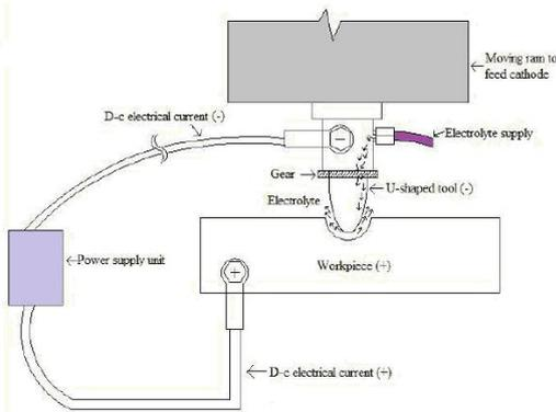
Figure 3.1: Principle of Electrochemical Machining
