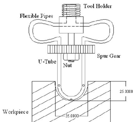
Figure 4.2: After Machining in step 2
