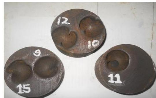
Figure 4.5: Work-piece after machining 9<sup>th</sup>, 10<sup>th</sup>, 11<sup>th</sup> and 12<sup>th</sup> run
