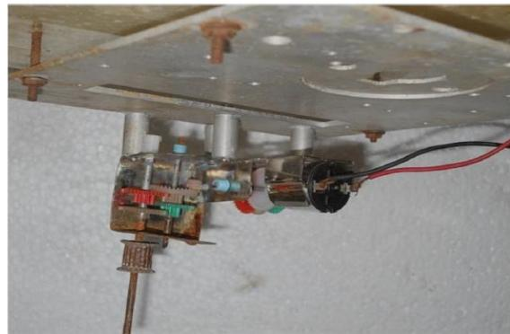
Figure 3.5: Reduction Gear box assembly fitted in ECM machine.
