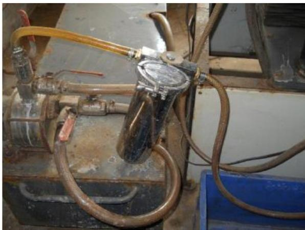
Figure 3.4 Electrolyte tank with Filter
