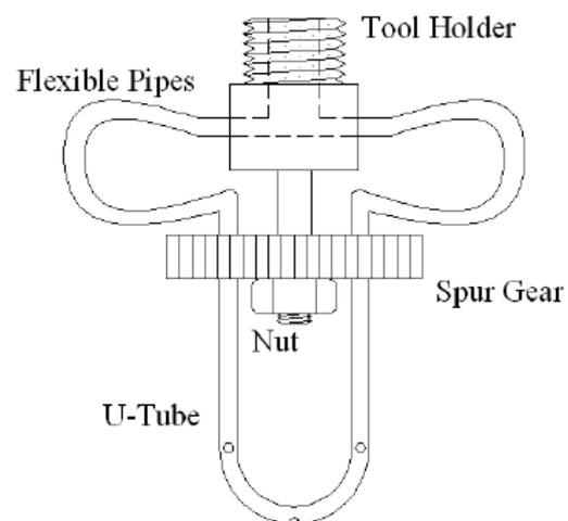
Figure 3.10: U-shaped Tool assembly
