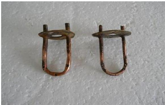
Figure 3.8: U-shaped Copper Tube
