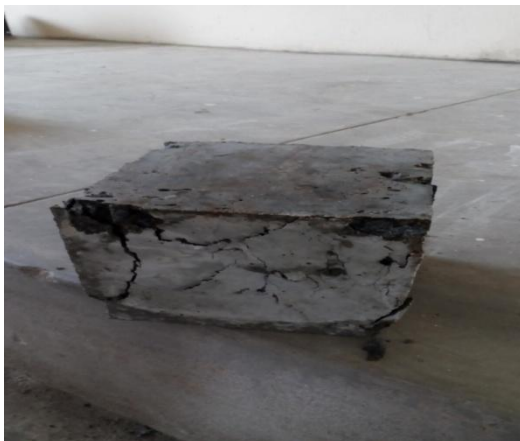
Fig (a): conventional concrete cube still with cracks after curing for 14days
