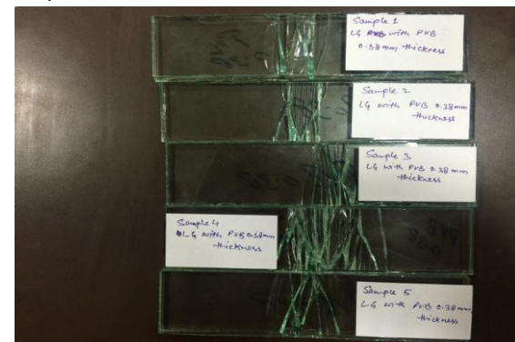
Fig No-7 PVB (0.38mm) Glass samples after test
