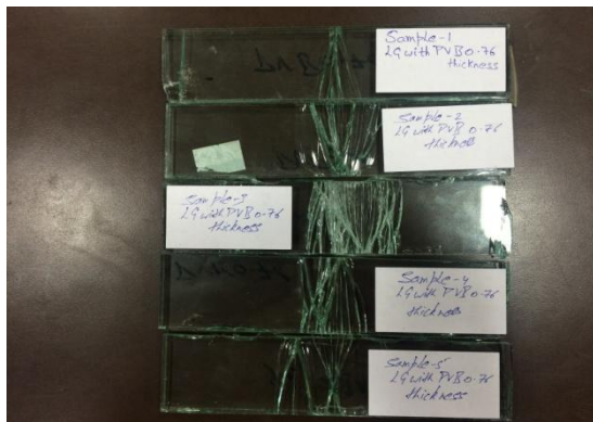
Fig No-9 PVB (0.76mm) Glass samples after test
