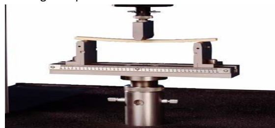
Fig No-3 Three-point bending test
