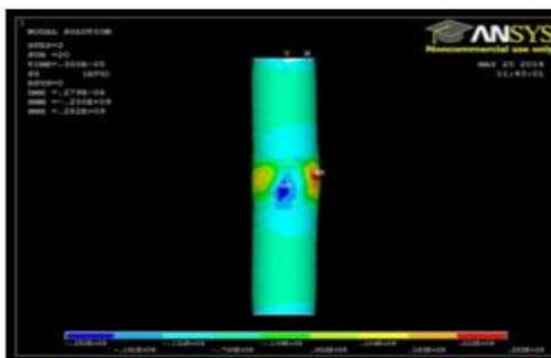
Fig. 23: Thermal Stress in Z-component at  $\text{ton}=0.52\mu\text{s}$
