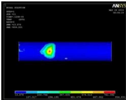
Fig.10: Temperature distribution in Brass wire with V=25V, I=27 A, P=0.38 and ton=1.2μs
