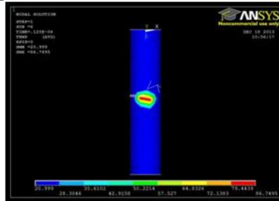
Fig5: Temperature distribution in Brass wire with V=25V, I=27 A, P=0.38 and ton=0.12μs
