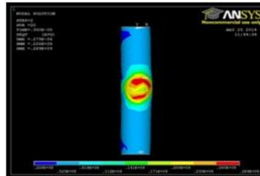
Fig. 26: Residual stress at toff =  $3\mu\text{s}$
