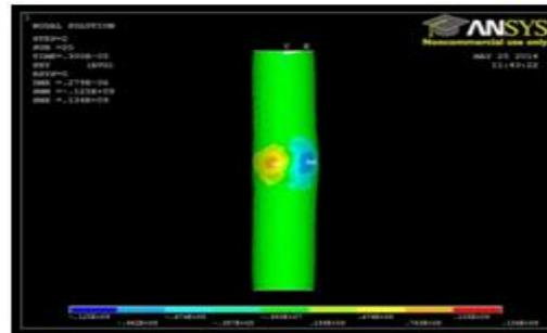
Fig. 24: Thermal shear stress in XY-component at  $\text{ton}=0.52\mu\text{s}$
