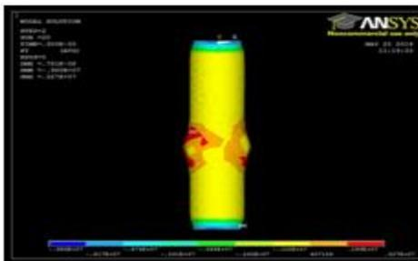
Fig. 14: Thermal Stress in X-component at  $t_{on}=0.12\mu s$
