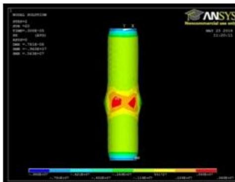
Fig. 15: Thermal Stress in Y-component at  $t_{on}=0.12\mu s$
