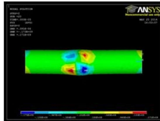
Fig. 32: Thermal Stress in YZ-component at ton=1.82μs
