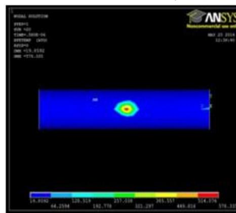
Fig.7: Temperature distribution in Brass wire with V=25V, I=27 A, P=0.38 and ton=0.36μs
