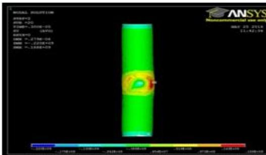
Fig. 22: Thermal Stress in Y-component at  $\text{ton}=0.52\mu\text{s}$
