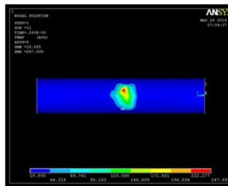
Fig.6: Temperature distribution in Brass wire with V=25V, I=27 A, P=0.38 and ton=0.26μs
