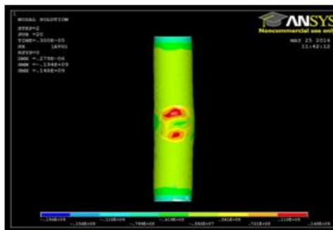
Fig. 21: Thermal Stress in X-component at  $\text{ton}=0.52\mu\text{s}$
