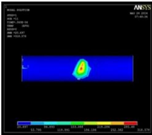
Fig.8: Temperature distribution in Brass wire with V=25V, I=27 A, P=0.38 and ton=0.58μs
