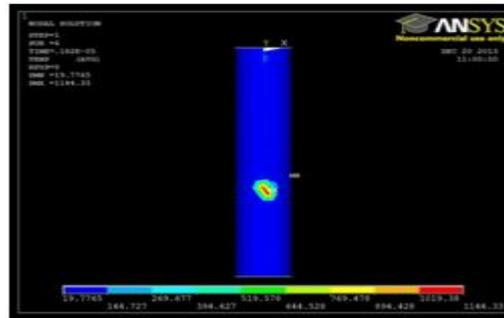
Fig. 11: Temperature distribution in Brass wire with V=25V, I=27 A, P=0.38 and ton= 1.82μs
