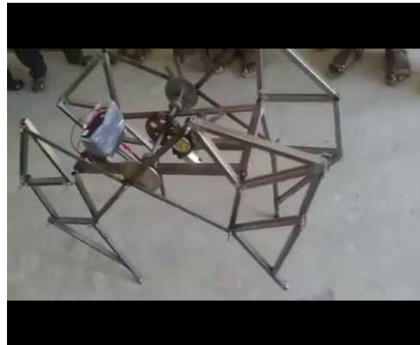
Fig.11- Theo Jansen four leg walking robot by using 8 bar mechanism
