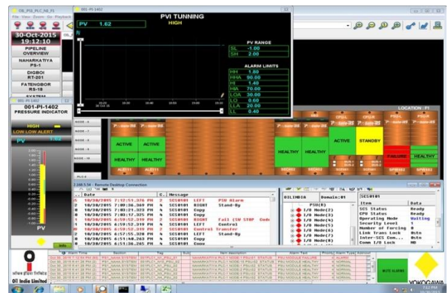
Figure 9: Graphic display of controller and I/O module status
