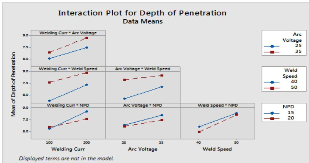
Fig 7. Interaction Plot for Depth of Penetration
