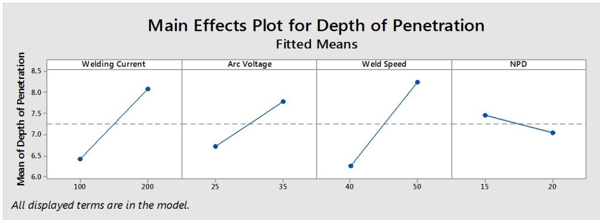
Fig 5. Main Effects Plot for Depth of penetration
