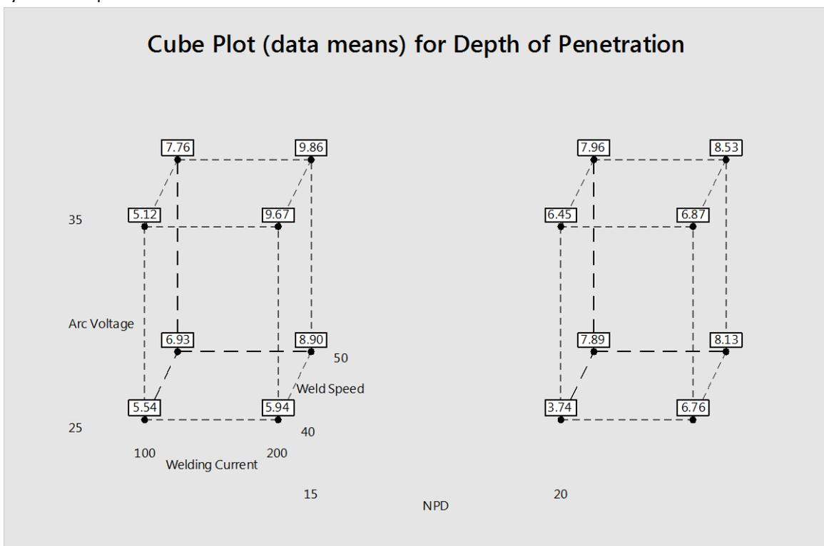
Fig2 The Geometric view of the Response variable Depth of Penetration
