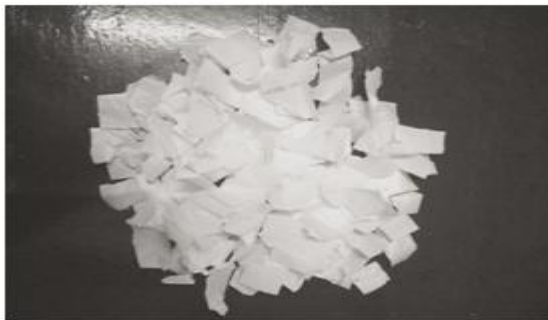
Fig : 2. Plastic Waste cut into strips of size(15*30)mm
