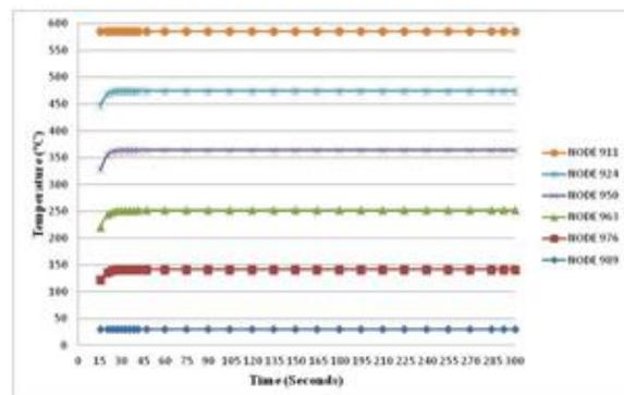
**Fig 4.6 Temperature variation with time along the c/s of slab**
