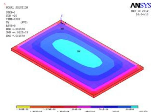
**Fig 4.17 Displacement considering both thermal and applied load**
