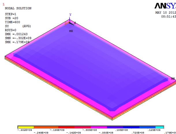
**Fig 4.12 Bending stress considering both thermal and applied load**
