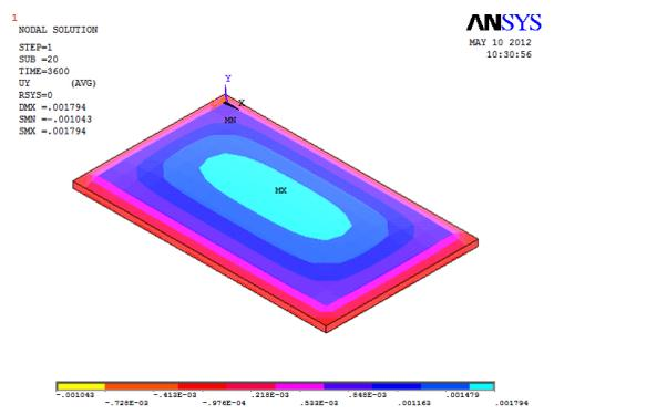
**Fig 4.21 Displacement considering both thermal and applied load**
