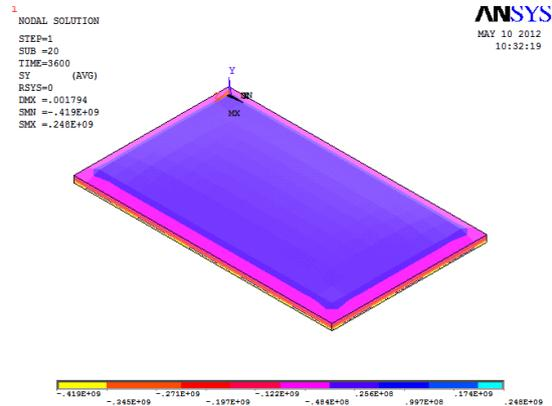
**Fig 4.24 Bending stress considering both thermal and applied load**
