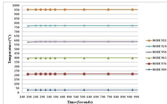
**Fig 4.22 Temperature variation with time along the c/s of slab**
