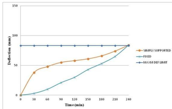
Fig 4.29 Post mid span downward deflection Vs fire exposure time
