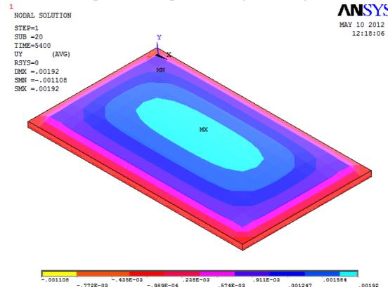
**Fig 4.25 Displacement considering both thermal and applied load**
