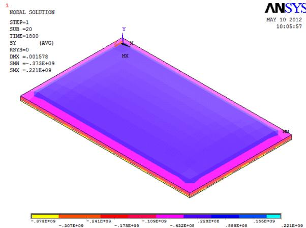
**Fig 4.20 Bending stress considering both thermal and applied load**
