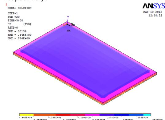
Fig 4.28 Bending stress considering both thermal and applied load
