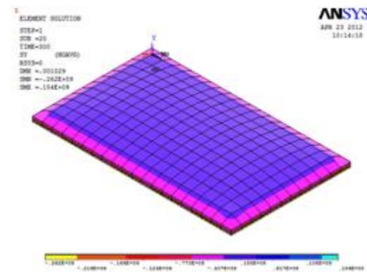
**Fig 4.5 Bending stress considering both thermal and applied load**
