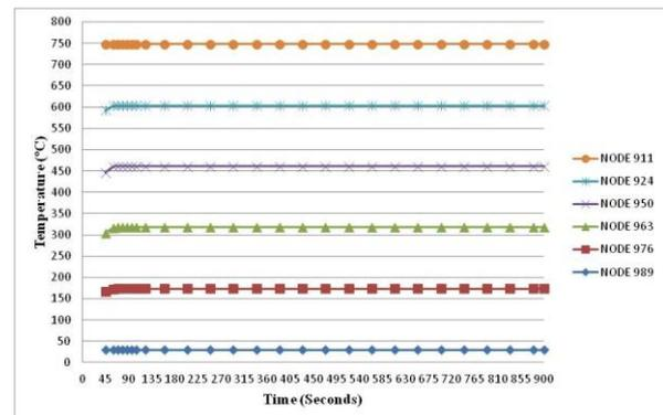
**Fig 4.14 Temperature variation with time along the c/s of slab**
