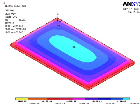
**Fig 4.13 Displacement considering both thermal and applied load**
