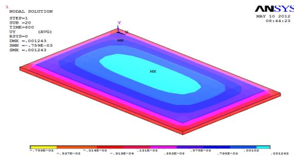
**Fig 4.9 Displacement considering both thermal and applied load**
