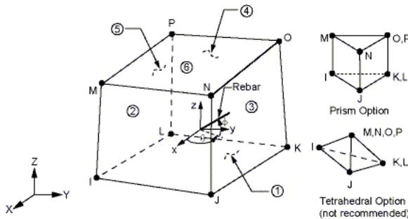
Fig 3.1 concrete element
