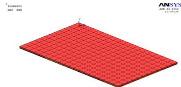
**Fig 4.1 Meshed Slab model**
