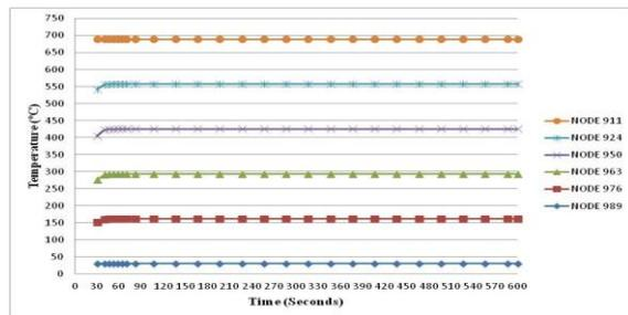
**Fig 4.10 Temperature variation with time along the c/s of slab**
