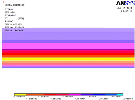
**Fig 4.16 Bending stress considering both thermal and applied load**
