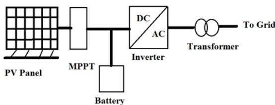
Figure 3: Schematic Diagram of a PV inverter for Grid Connected Operation.
