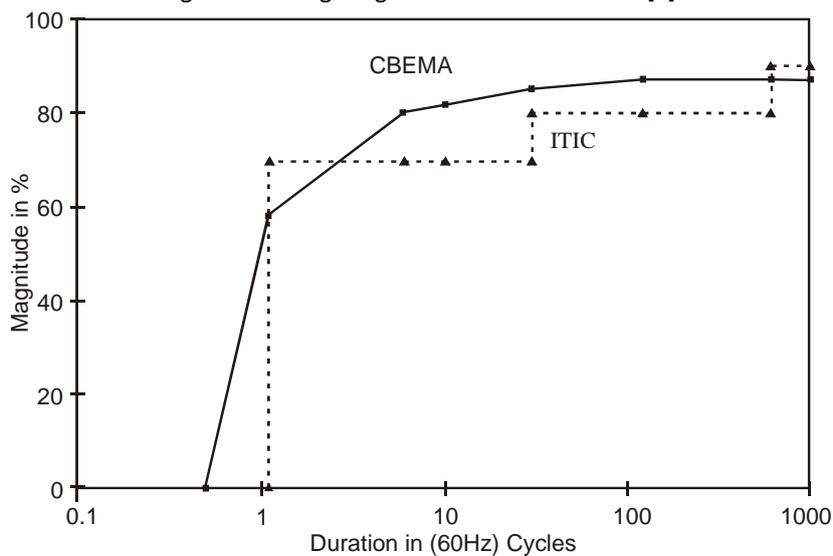
Figure 2: CBEMA and ITIC curve [8]
