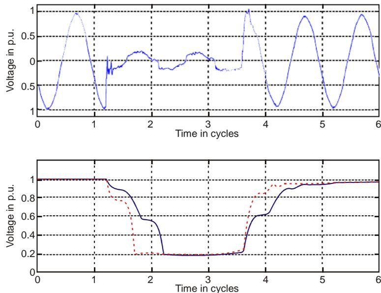
Figure 1: Voltage sags and its characteristics [7]
