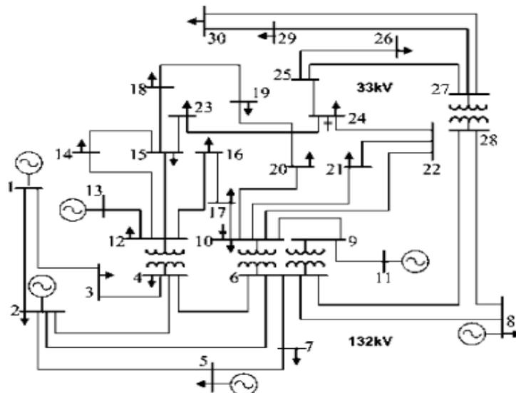
Figure 4: Single-line diagram of the IEEE-30 bus system[21].
