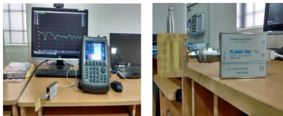
Fig.4 Experimental setup for proposed antenna
