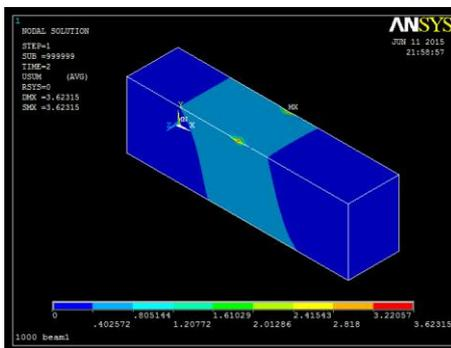
Fig.4.17 (b) Deflection contour plot of beam with reinforcement with 15624 number of elements
