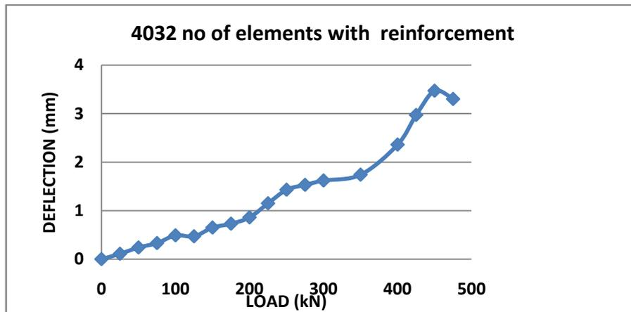
Fig 4.24 variation of deflection with load for the beam with reinforcement having 4032 number of elements
