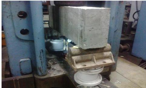
Fig.4.3 RCC Beam placed in UTM for testing
