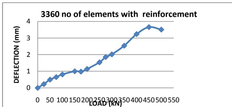
Fig 4.26 variation of deflection with load for the beam with reinforcement having 3360 number of elements
