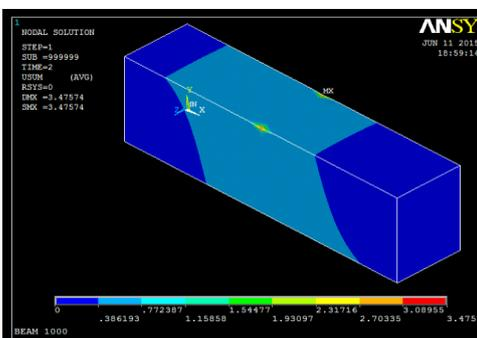
Fig. 4.16(b) Deflection contour plot of beam with reinforcement with 4032 number of elements
