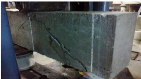
Fig.4.4 crack developed in the RCC beam subjected to loading
