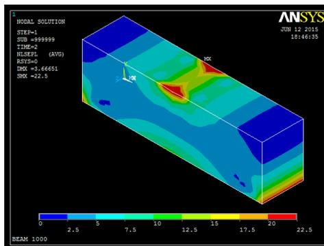
Fig. 4.18(b) Von mises stress contour plot of beam with reinforcement of 3360 number of elements
