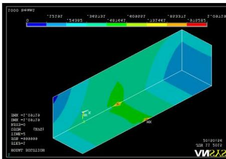
Fig.4.17 (a) Deflection contour plot of beam with reinforcement with 15624 number of elements
