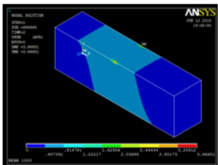
Fig. 4.15(b) Deflection contour plot of beam with reinforcement with 3360 number of elements
