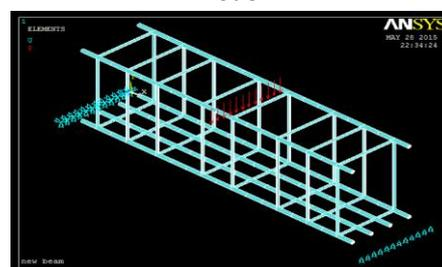
Figs 4.14(a) showing the loading conditions of beam model with reinforcement
