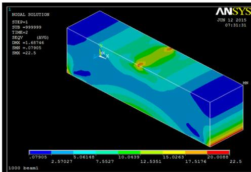
Fig. 4.18(a) Von mises stress contour plot of beam without reinforcement with 3360 number of elements
