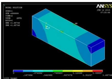
Fig. 4.15(a) Deflection contour plot of beam without reinforcement with 3360 number of elements
