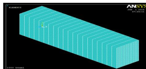
Fig 4.9 Beam model with 15624 mesh elements
