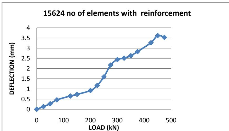
Fig 4.22 variation of deflection with load for the beam with reinforcement having 15624 number of elements
