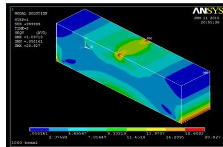
Fig.4.20 (a) Von mises stress contour plot of beam without reinforcement with 15624 number of elements
