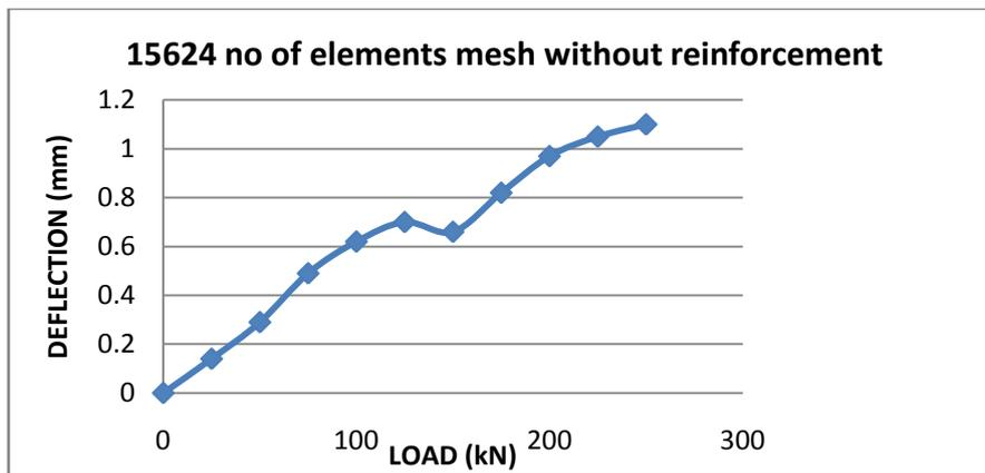
Fig.4.21 variation of deflection with load for the beam without reinforcement having 15624 number of elements
