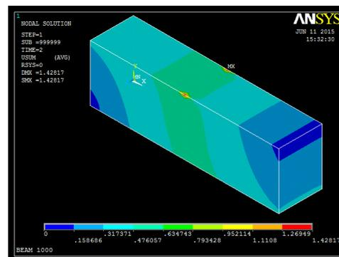
Fig. 4.16(a) Deflection contour plot of beam without reinforcement with 4032 number of elements
