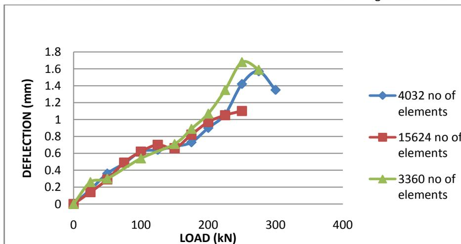
Fig.4.27 variation of deflection with load for the beams without reinforcement having different number of elements
