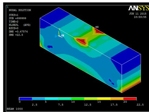
Fig 4.19(b) Von mises stress contour plot of beam with reinforcement with 4032 number of elements
