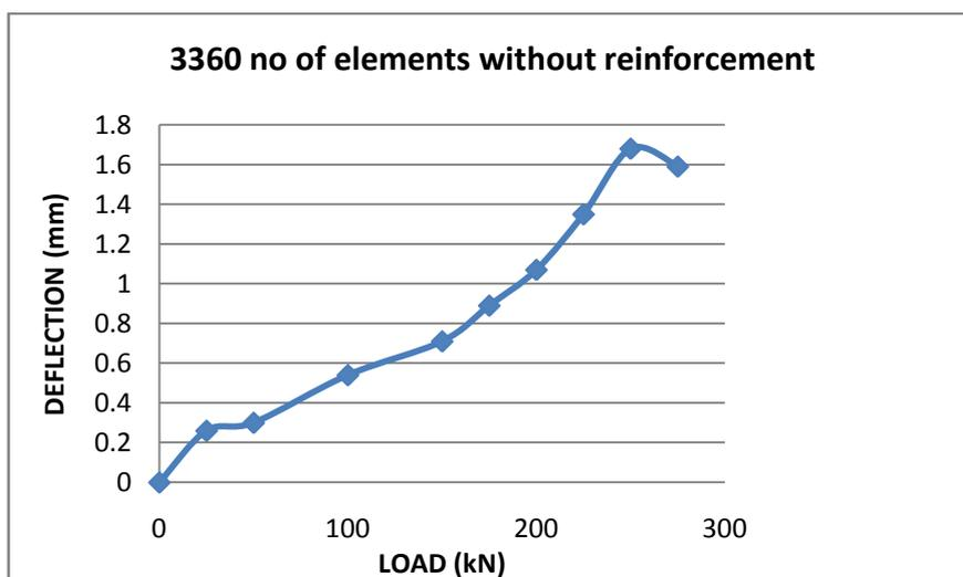
Fig 4.25 variation of deflection with load for the beam without reinforcement having 3360 number of elements
