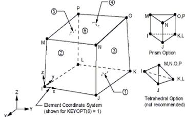
**Fig 4.5 Element Solid65 3-D reinforced concrete**
