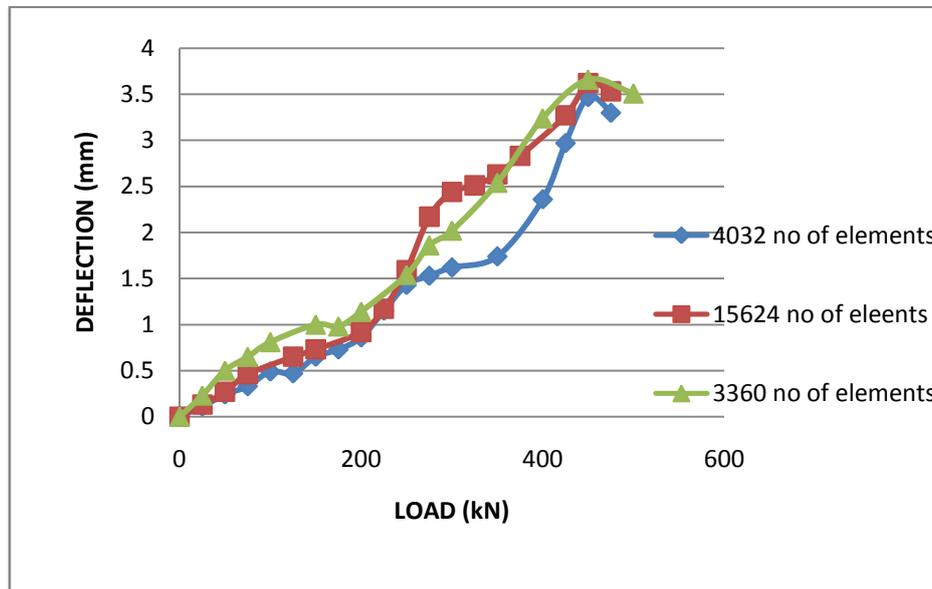
Fig.4.28 variation of deflection with load for the beams with reinforcement having different number of elements
