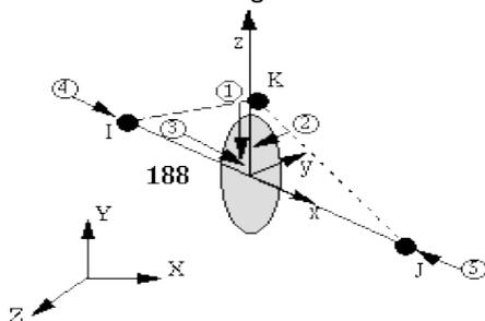
**Fig 4.6 Beam 188 3-D spar element**
