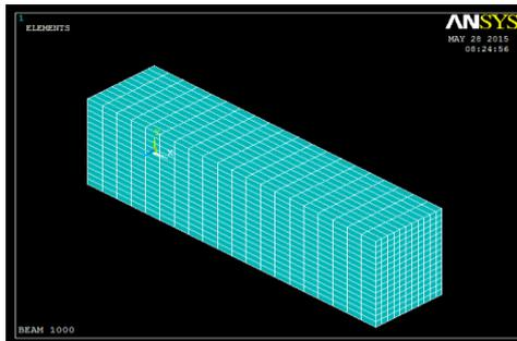
Fig 4.10 Beam model with 4032 mesh elements
