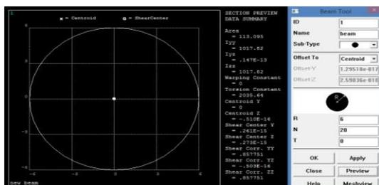
Fig 4.7 showing the sectional properties of the reinforcement
