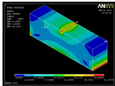
Fig. 4.19(a) Von mises stress contour plot of beam without reinforcement with 4032 number of elements
