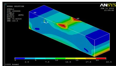
Fig. 4.20(b) Von mises stress contour plot of beam with reinforcement with 15624 number of elements
