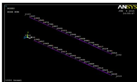
Fig 4.12(a) Meshing of longitudinal reinforcement
