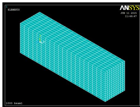
Fig 4.11 Beam model with 3360 mesh elements
