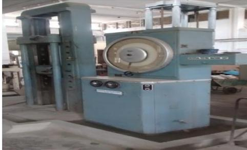
Fig.4.1. Universal Testing Machine
