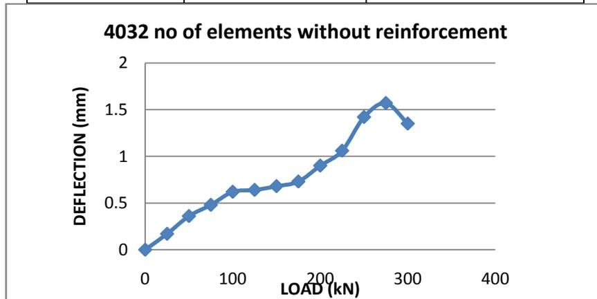
Fig 4.23 variation of deflection with load for the beam without reinforcement having 4032 number of elements
