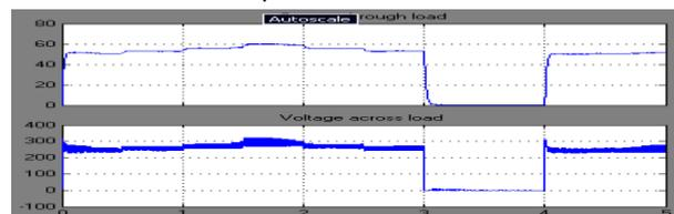
**Fig 21: current and voltage near DC load with PV cell interruption between 3 to 4 seconds without battery backup**
