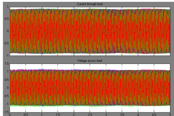
**Fig 9: current and voltage at AC load without MPPT algorithm**
