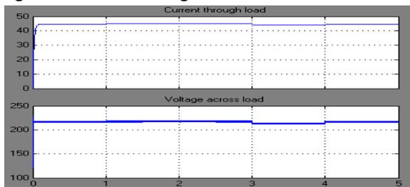
**Fig 24: current and voltage near DC load with PV cell interruption between 3 to 4 seconds without battery backup**
