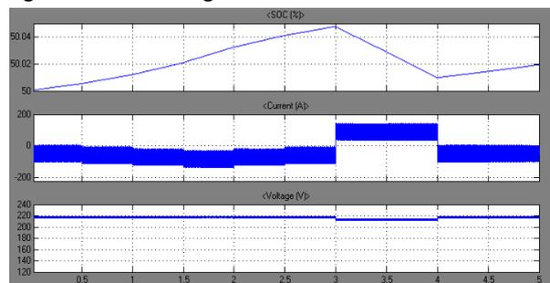
**Fig 27: %SOC, Current and Voltage of battery when PV cell fails between 3 to 4 seconds**
