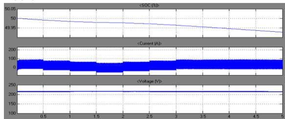
**Fig 11: Battery SOC %, current and voltage without MPPT algorithm**
