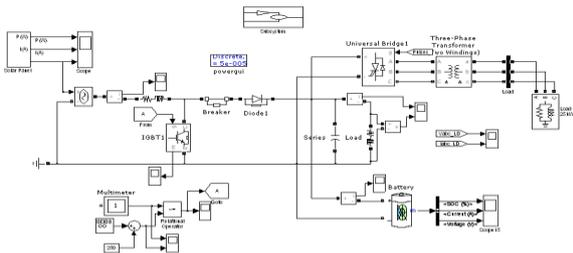
**Fig 6: PV module with battery backup for AC and DC load**
