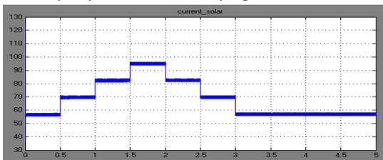
**Fig 7: shows the current through the solar power, variation is due to disparity in solar irradiation without MPPT algorithm.**
