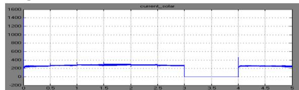
**Fig 20: current through solar cell with its interruption between 3 to 4 seconds without battery backup**
