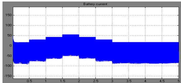
**Fig 10: Battery current without MPPT algorithm**
