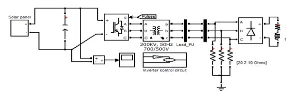
**Fig.32 Simulink diagram of PV inverter for distorted and unbalanced load.**
