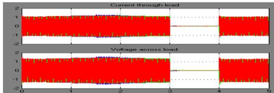
**Fig 22: current and voltage near AC load with PV cell interruption between 3 to 4 seconds without battery backup.**
