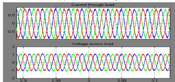
**Fig 26: Zoomed view of current and voltage near AC load with PV cell interruption between 3 to 4 seconds without battery backup**
