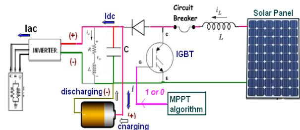
**Fig 1: Block diagram representation of PV-battery system with AC and DC Loads**
