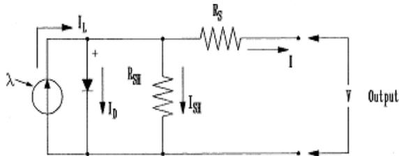
**Fig 2. Equivalent electrical circuit of pv module, showing the diode and ground leakage currents.**
