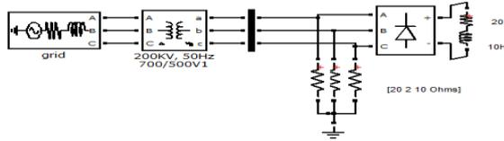
**Fig.28 Simulink diagram of grid circuit for distorted and unbalanced load.**
