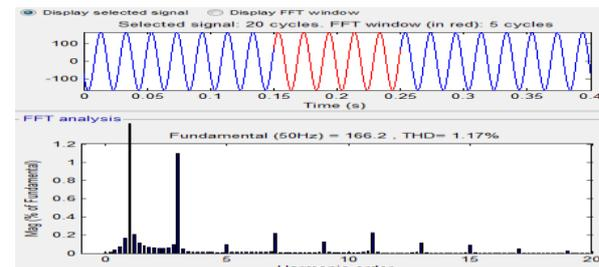
**Fig. 31 THD of blue color waveform for grid connected load current**
