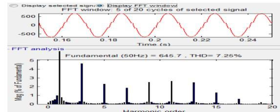
**Fig. 30 THD of blue color waveform for grid connected load voltage**
