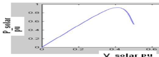
Fig3a: Shows P-V characteristics of solar cell with constant irradiation
