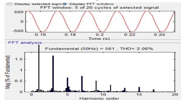
**Fig. 36 THD of blue color waveform for inverter connected load voltage**
