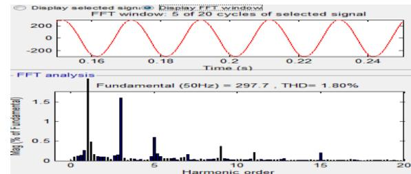
**Fig. 37 THD of blue color waveform for inverter connected load current**
