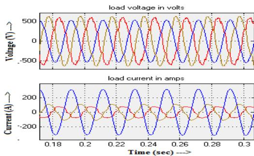
**Fig.33 Load voltage and current waveforms for PV inverter circuit**
