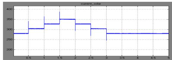
**Fig 12: current output from solar cell with MPPT algorithm**
