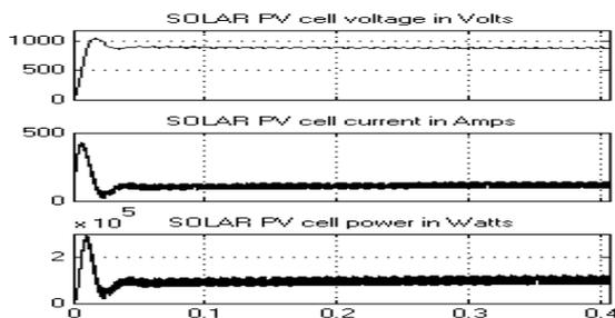
**Fig.34 solar PV cell output voltage, current and power waveforms**
