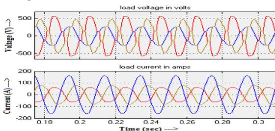
**Fig.29 Load voltage and current waveforms for grid supply circuit**
