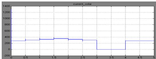
**Fig 23: current through solar cell with its interruption between 3 to 4 seconds with battery backup**
