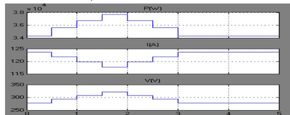
**Fig 13: solar cell output power, current and voltage under normal conditions with MPPT algorithm**
