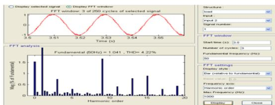
**Fig 18: voltage THD with MPPT algorithm for 3 cycles taken at 3.5 seconds**
