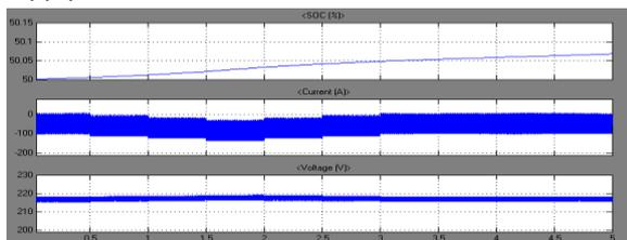
**Fig 17: Battery SOC %, current and voltage with MPPT algorithm**
