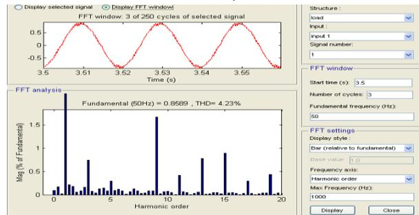
**Fig 19: current THD with MPPT algorithm for 3 cycles taken at 3.5 seconds**
