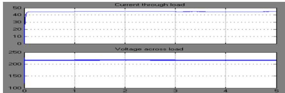
**Fig 16: current and voltage at DC load with MPPT algorithm**
