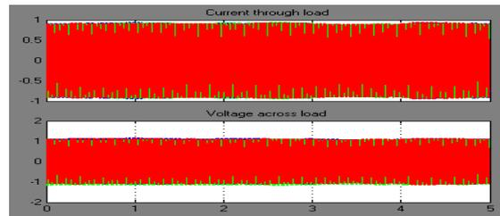
**Fig 25: current and voltage near AC load with PV cell interruption between 3 to 4 seconds with battery backup**
