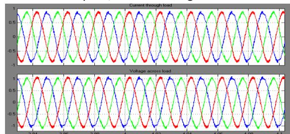
**Fig 9: Zoomed view of current and voltage at AC load without MPPT algorithm**
