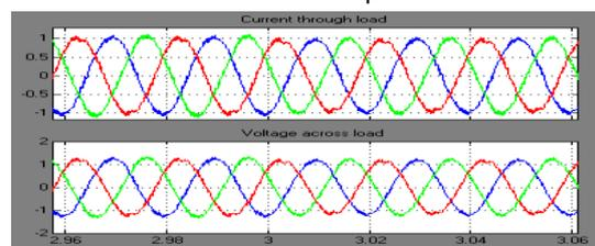
**Fig 15: Zoomed view of current and voltage near AC load under normal conditions with MPPT algorithm**
