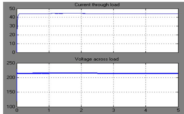
**Fig 8: current and voltage near DC load without MPPT algorithm**
