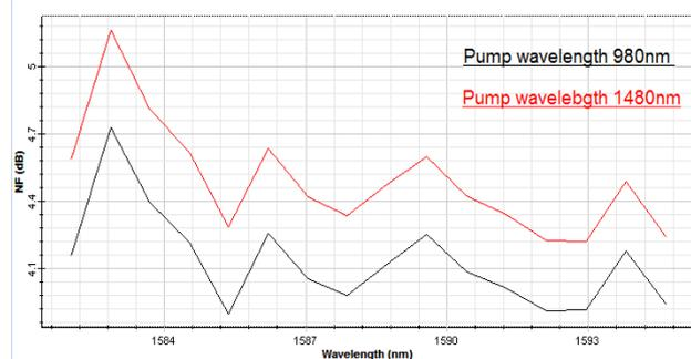
Figure4. Noise figure vs Wavelength
