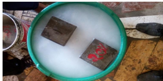
Figure 6 Aid curing of concrete cubes
