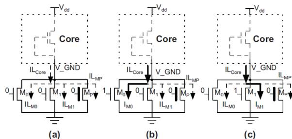
**Fig.3.** Proposed architecture: (a) snore mode, (b) dream mode, (c) sleep mode.
