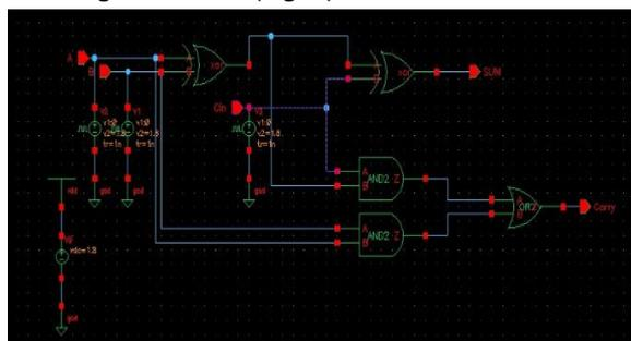
**Fig.8.** Schematic of Full Adder using Cadence
