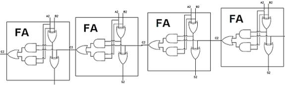
**Fig.7.** 4-bit Ripple Carry adder
