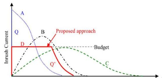
Fig.1. Tradeoff of inrush current and the expected current budget control.
