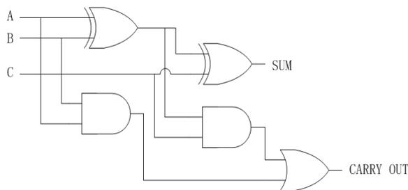
**Fig.6.** Gate level Diagram of Full Adder
