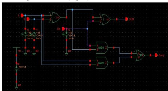
**Fig.8.** Schematic of Full Adder using Cadence
