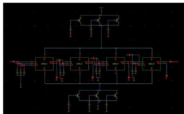
**Fig.10.** Schematic of 4-Bit Adder using Cadence with MTCMOS
