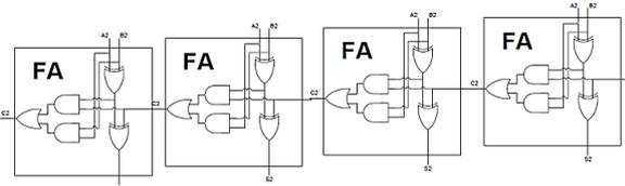
**Fig.7.** 4-bit Ripple Carry adder
