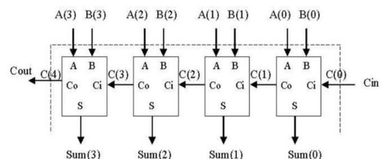
**Fig.4.** 4 Bit Adder
