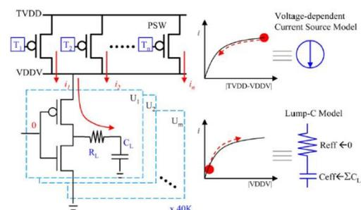
Fig.2. Power ramp-up and effective capacitance modeling.
