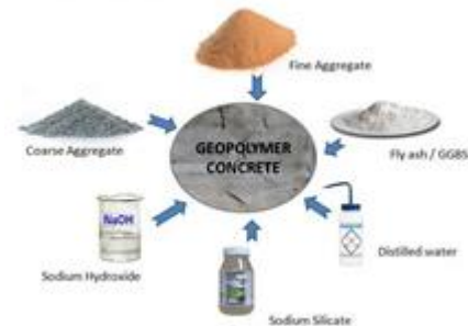
Fig -8: Constituents in Mix Design of Geo Polymer Concrete
