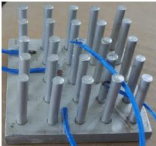
Fig.2 Pin Fin Heat sinks with thermocouples
