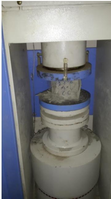
Figure showing Compressive testing machine SPLIT TENSILE STRENGTH:
