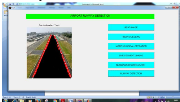
Fig. 21 Output of runway detection (red lines).
