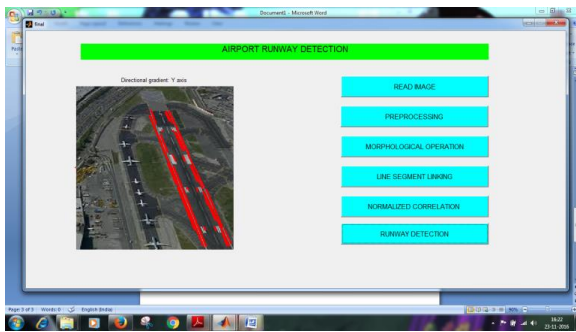
Fig 11. Output of runway detection (red lines).
