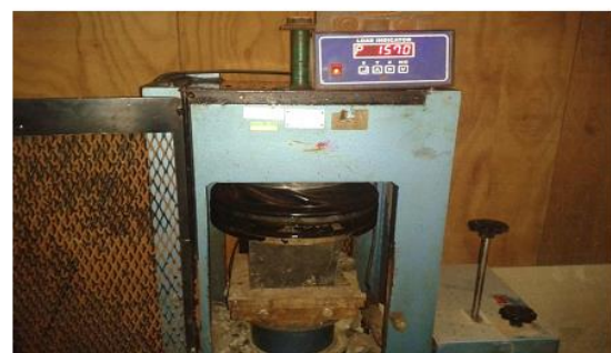
Figure 5 Test setup of compressive strength
