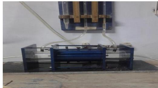
Hole Erosion Test(HET) apparatus (without water circulation)
