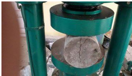
Figure 8.3: Picture shows the Split tensile strength
