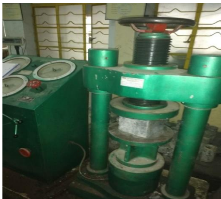
Figure 8.1: Picture showing the compressive testing for cubes
