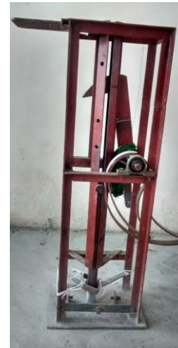
Fig. 1.0 Schruder’s impact testing machine- A fabricated equipment
