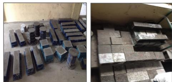
Figure 2. Casting and curing of specimens
