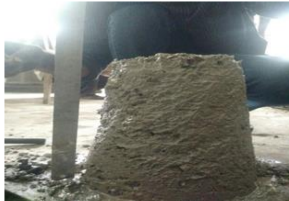
Figure 3.3: Flow of slump after release
