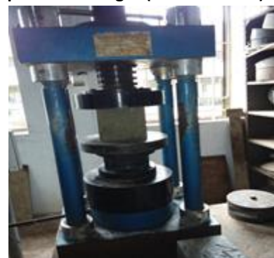
Fig 3.1 : compressive strength testing machine
