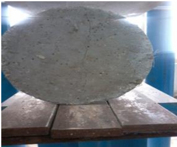
Fig 3.2: Split Tensile test on Cylinder
