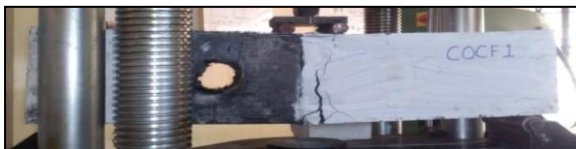
Fig. 9. Crack pattern of beam with opening strengthened using CFRP sheets
