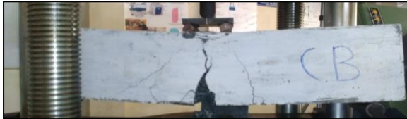
Fig. 6. Crack pattern of Control beam without opening CB
