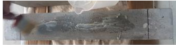
Fig. 5 Application of epoxy resin
