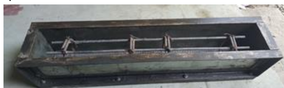
Fig. 3 Mould used for casting beams
