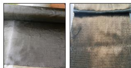
(a) CFRP sheet (b) BFRP sheet
