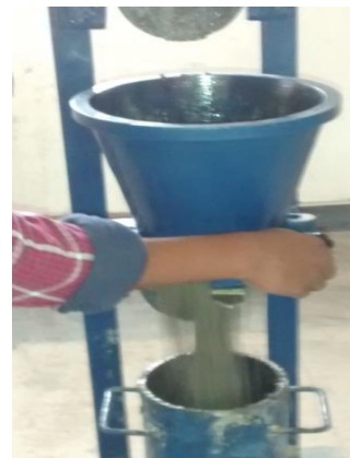
Fig -2: Compaction Factor Test
