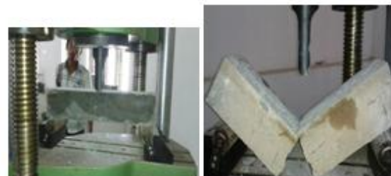
Fig -5: Beam Under Tension and Beam after Failure
