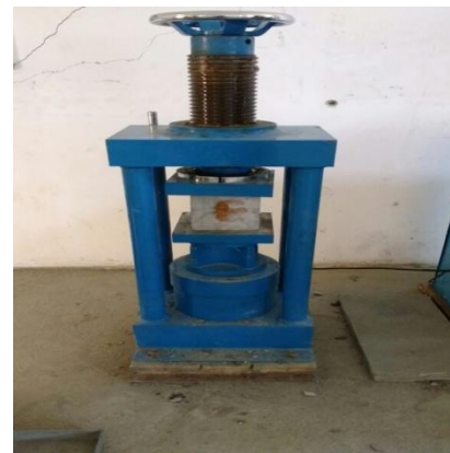
Fig -4: Cube test under Compression
