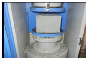
Fig.5.1. Compressive strength testing
