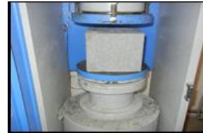
Fig.5.1. Compressive strength testing
