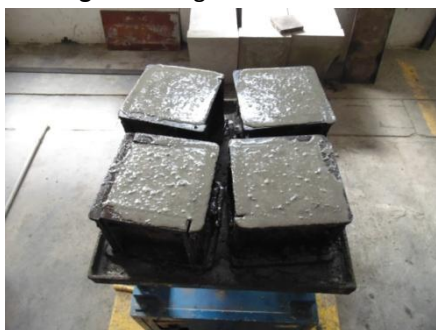
Fig -6: Cube moulds on vibratory machine
