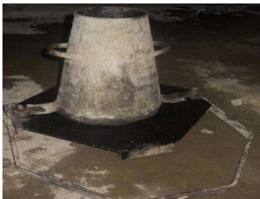
Fig -3: Slump cone apparatus
