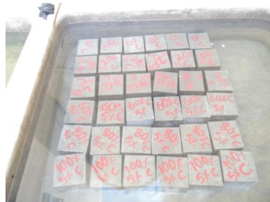
Fig -7: Curing of Concrete specimens in water
