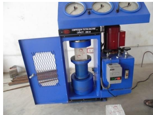
Fig -8: Testing of concrete specimen.
