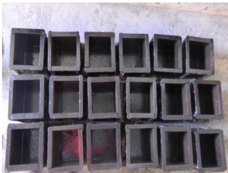
Fig -4: Cube moulds ready to use
